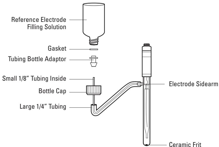
5. Remove the cap and fluid seal from reference electrode fill solution bottle (Cat. No. 181073). Hold the bottle in an upright position. Check that the rubber gasket is properly aligned, and then connect the cap end of the tubing assembly to the bottle. The 1/8 inch tubing should extend into the bottle.
