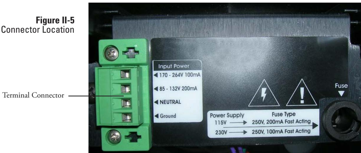
5. Wire the power cable to the green screw terminal connector from the options kit. Select correct terminal for hot conductor depending on line voltage. Refer to **Figure II-5** for terminal connector location.
