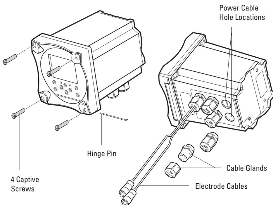
1. Open the faceplate – loosen the four screws using a Phillips head screwdriver. The electronics faceplate will open via the hinge pin connection.
