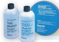
**Total Alkalinity Test Kit:** A two-step direct measurement of total alkalinity and pH. Calibrate for pH, add alkalinity reagent and read total alkalinity of 0-200 ppm CaCO<sub>3</sub> from the included pH conversion chart.
