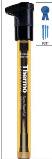
**Single Junction Sure-Flow® reference half-cell with epoxy body**
