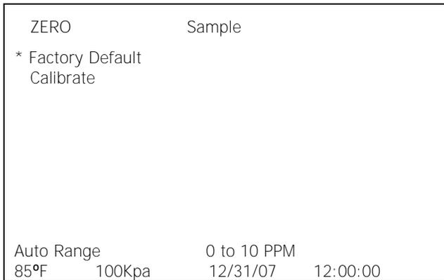
Advance the cursor (\*) to the Factory Default Zero option and press ENTER. Within seconds the system returns to the MAIN MENU in the "Sample" mode.
