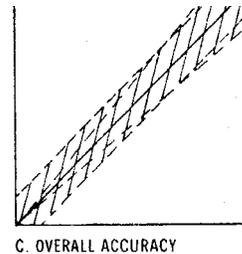
**Example 1:** As illustrated by Graph A any error, play in the multi-turn span pot or the temperature compensation circuit, during a span adjustment at 20.9% (air) of full scale range would be multiplied by a factor of 4.78 (100/20.9) if used for measurements of 95-100% oxygen concentrations. Conversely, an error during a span adjustment at 100% of full scale range is reduced proportionately for measurements of lower oxygen concentrations.
