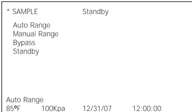
The analyzer is equipped with five (5) standard measuring ranges (see specification) and provides users with a choice of sampling modes. By accessing the MAIN MENU, users may select either the Auto Range or a fixed Manual Range) mode.
