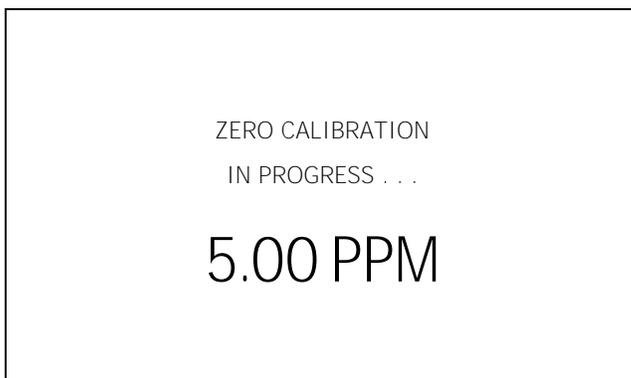
After the oxygen reading has stabilized, press ENTER to complete the Zero Calibration. If the user attempts to initiate the ZERO CALIBRATION function while the oxygen reading is above 50% of the most sensitive or lowest range, the system displays the message "CALIBRATION FAILED" and returns to the "Sample" mode.
