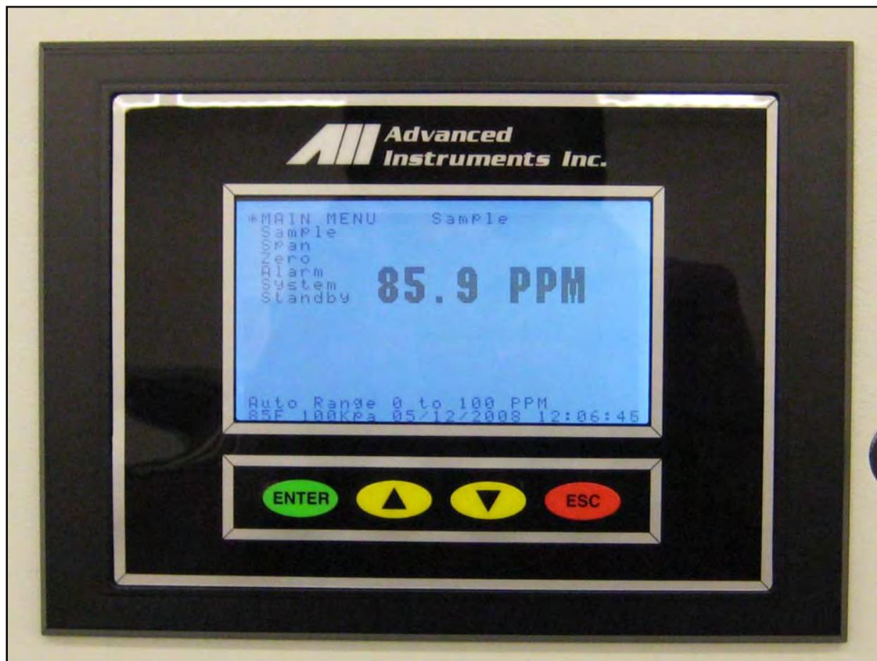
Note: In the event power to the analyzer is interrupted, the system defaults to the "Standby" mode when power is restored. To resume sampling, advance the cursor (\*) to "Sample" mode, press ENTER to select and select the range mode as described below.
