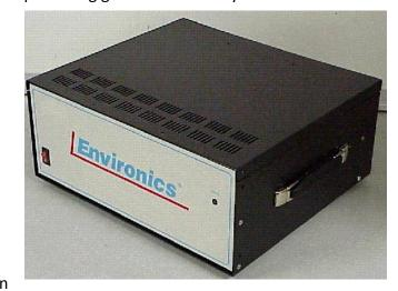
The Series 4020 consists of a single chassis supporting up to four mass flow controllers. The mass flow controllers are factory calibrated using a primary flow standard traceable to the United States National Institute of Standards and Technology (NIST). Each flow controller utilizes an 11 point calibration table with linear interpolation, to increase accuracy and reduce flow controller nonlinearity.
