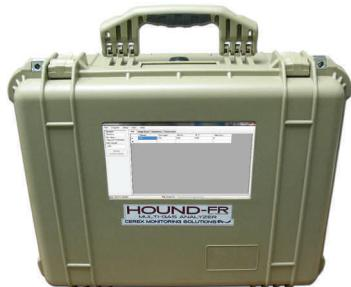
**Hound-FR:** Our largest and most sensitive model. This analyzer is equipped with sealed external LAN (1), WAN (1) and USB (1) ports as well as two internal USB ports for simple installation of USB peripheral devices such as cellular modem, GPS or streaming web camera. This unit offers excellent detection limits with a 17 meter sample path and is equipped with wheels for rolling transport: 38 Lbs.
