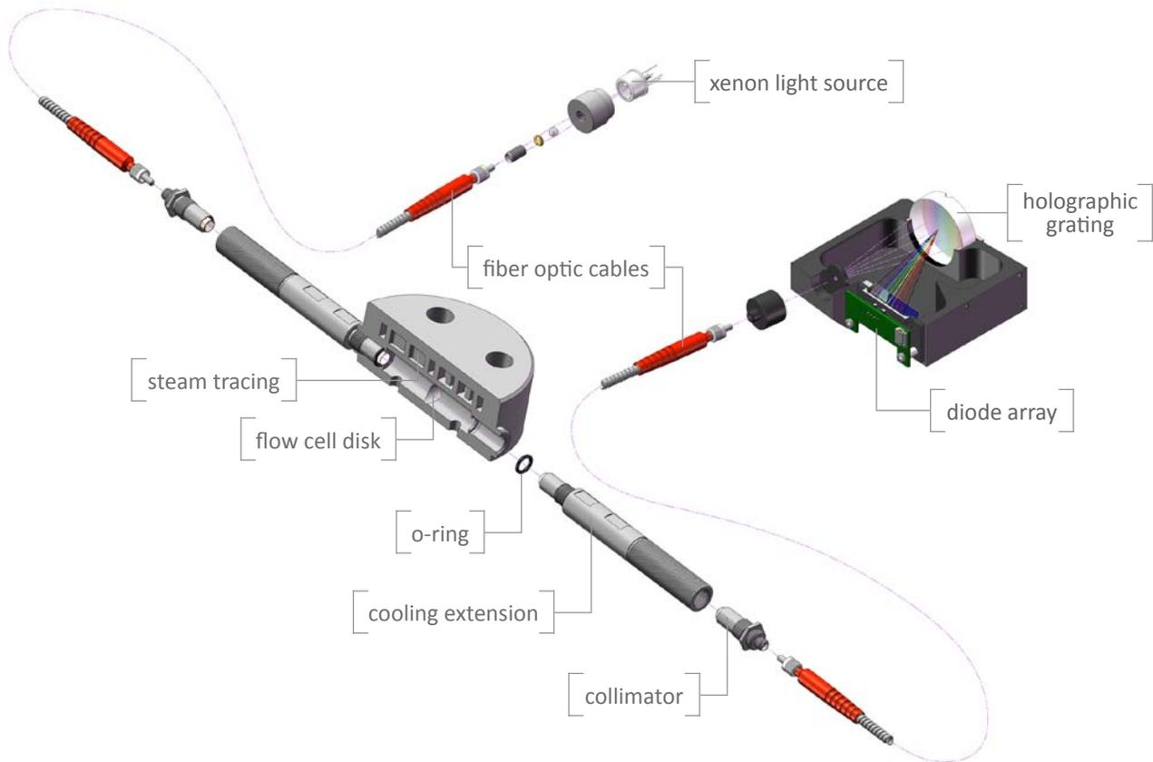
The signal originates in the pulsed xenon light source and travels via fiber optic cable to the flow cell disk, which is built into the head of the probe. Passing through the length of the flow cell, the signal picks up the absorbance imprint of the continuously drawn sample gas.
