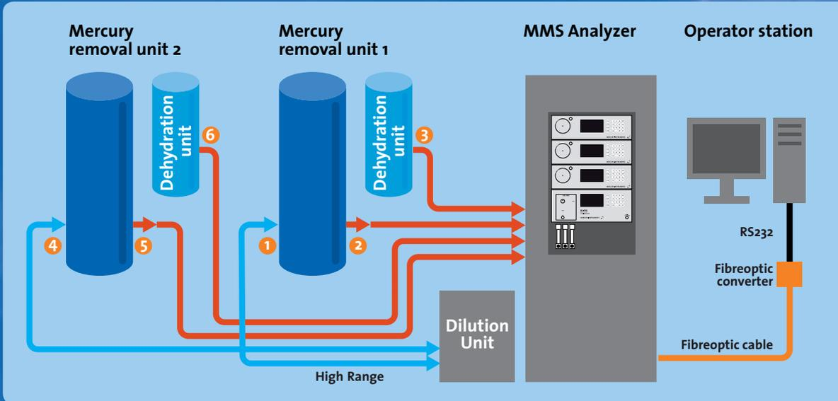
Example: the MMS Mercury Monitoring System installed in a gas separation plant, where mercury must be removed from the gas to avoid corrosion of aluminum heat exchangers and to produce mercury-free product streams. The MMS is the perfect tool to monitor the efficiency of the mercury removal units and to verify a low mercury concentration in the processed gas.
