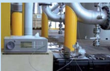
On-line field measurement of mercury in a natural gas plant. This mobile setup employs a SCS and a UT-3000 Mercury Ultratracer. The result: quick measurement of the mercury load of the gas at different points and its distribution in the process.
