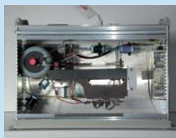
Automatic calibration unit. The system is based on mercury concentration in a saturation chamber. This concentration is automatically calculated using the mercury vapor pressure equation according to NIST.
