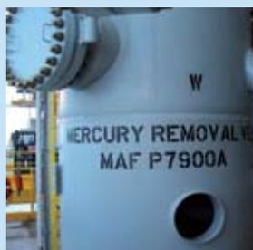
A Mercury Removal Unit (MRU) on an offshore platform. The MRU reduces the mercury in a natural gas stream via a bed of sulfurized activated carbon. The mercury concentration at the outlet is monitored to be less than 10  $\text{ng}/\text{m}^3$ ; this level is regarded as harmless to plant components downstream.
