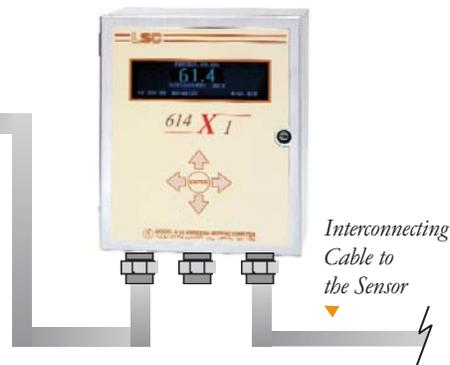
The Model 614 has the ability to change calibration files from a remote location by incorporating the LSC 614 Remote Control Box. This control box contains its own display that provides the customer with the process measurement and temperature. It can be located up to 3 km. away, via the 2 wire RS-485 connection. The zero offset can also be changed from the remote enclosure.
